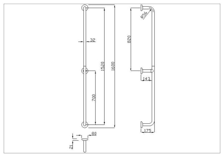
Wall-to-wall grab bar made of steel pipe, painted with synthetic thermoplastic powder of plant origin, Rilsan®
